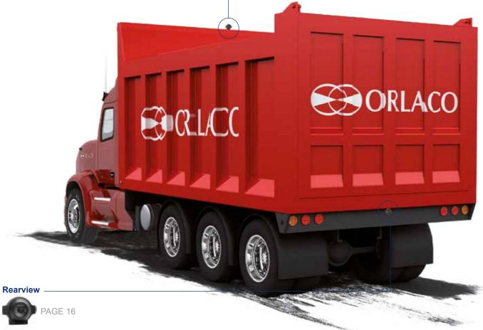
The Rearview camera lets you see the area directly behind the truck. The monitor in the cab automatically switches over to this camera view if you select a reverse gear, allowing you to reverse safely.
